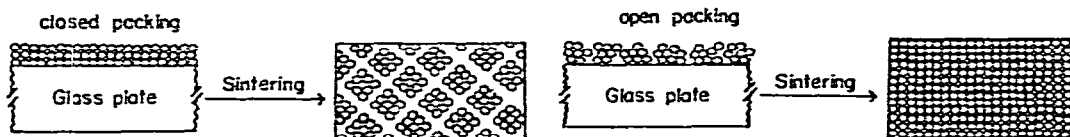
Fig. 11. Schematic diagram of structure of silica gel and borosilicate glass powder before and after sintering.
